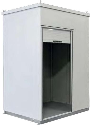
The CLASSIC construction is a proven system with a unique C-rail concept. Here, the weight of the fixtures is transferred to the corner posts made of high-strength pulltruded profiles. Thanks to the proven sandwich construction of [GRP \(pg. 11\)](#) and rigid polyurethane foam core, this series also features very good thermal insulation.
