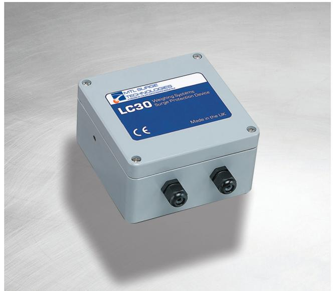
**The LC30 surge protection device protects load cell and weighing system installations from possible malfunctions** or damage to individual strain-gauge bridges of associated electronic instrumentation etc. caused by severe overvoltages or impulse currents on signal cabling.
